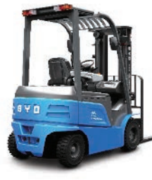
ECB20 Load capacity: 2.0 ton Service weight: 3,600 kg Min. turning radius: 2,020 mm Voltage: 80 V Battery capacity: 270Ah/540Ah
